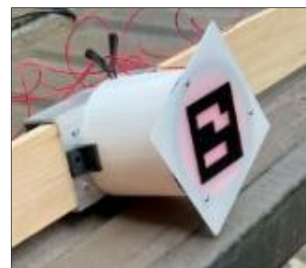
Figure 4: Assembled light marker
